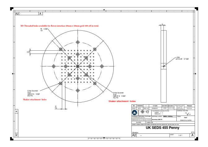
Figure E-1: RAL Space Vibration interface plate
