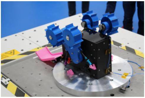
Figure D-4: Vibration Testbench Setup
