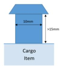
Figure E-3: The Cylindrical Peg cargo interface
