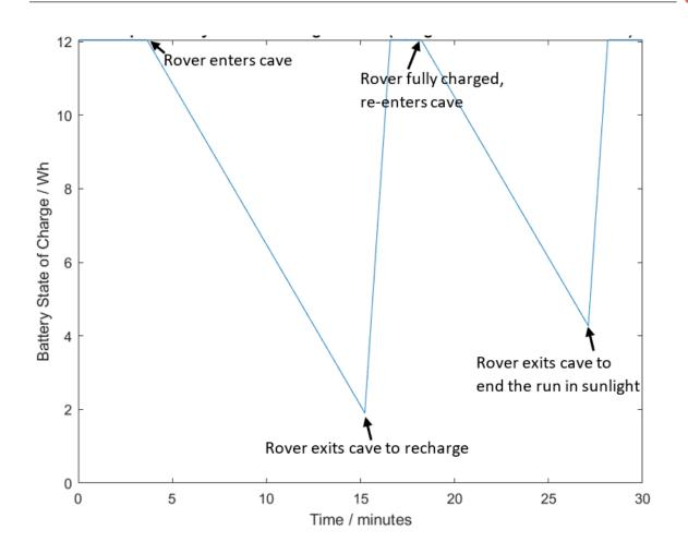
Figure 2-1: Example Battery State of Charge Profile (3.5kg Rover with 5 Sparkwing Solar Panels)
