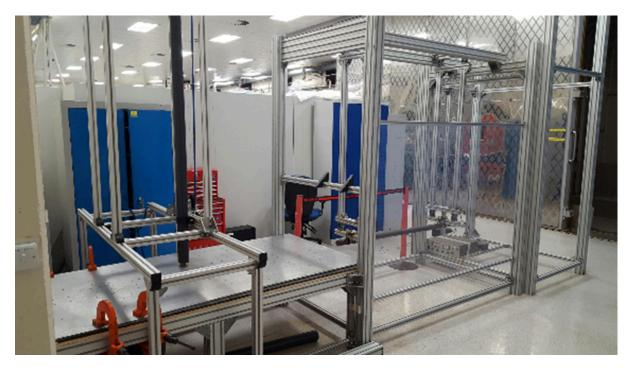
Figure D-5: Shock Test Setup
