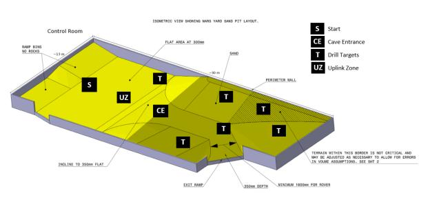
Figure D-3: Airbus D&S Mars Yard - Topology Schematic - (Light and dark side of cave, with start, cave entrance and uplink zone shown. Drill target site locations demonstrated - these may change on the day)
